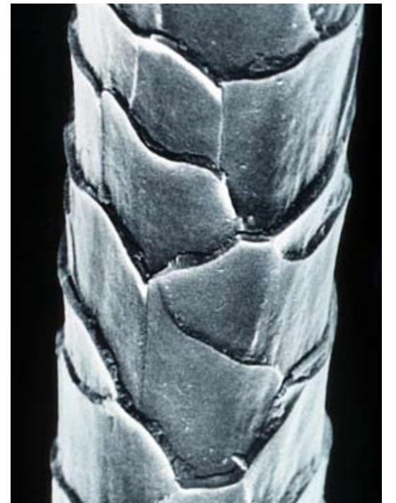
A microscopic view of a wool fibre showing its surface scales
